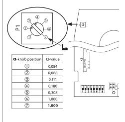
In order to have optimal control, linear characteristics of system (valve, actuator, HEX) is required. This can be assured using the right  $\alpha$  value. Appropriate  $\alpha$  value depends on temperatures of heating/cooling medium and controlled temperature of heated/cooled medium. Calculate  $\alpha$  value according to the Tech Note number VNHUA102 (Setting the right  $\alpha$  value).
